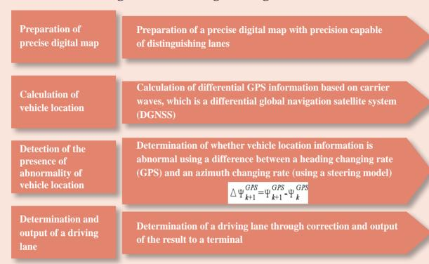
According to a method of determining a driving lane using a steering model, when abrupt tolerance occurs and a driving lane is inappropriately recognized in matching of lanes for distinguishing lanes, a heading changing rate and a location changing rate of a vehicle are compared using a vehicle dynamics model, and therefore a driving lane of an actual vehicle is matched.
